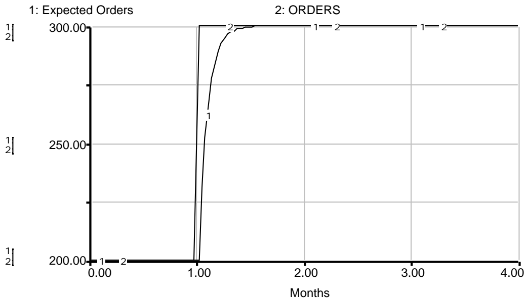
Figure 8: Behavior of the model with DT = 0.03125 months and “TIME TO CHANGE EXPECTATIONS” = 0.1 months
